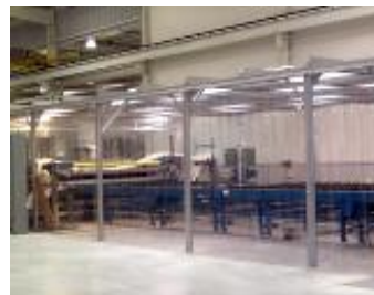
Modular cleanroom enclosures can typically be reconfigured, relocated and re-certified for re-designated usage. Photos courtesy of Simplex Isolation Systems.
