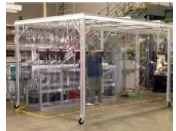
Modular cleanroom enclosures can typically be reconfigured, relocated and re-certified for re-designated usage. Photos courtesy of Simplex Isolation Systems.
